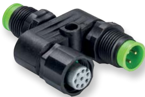
STS-CON-488 T-Connector for the extraction of the diagnostic output or coupling a restart signal into the switch (optional)
